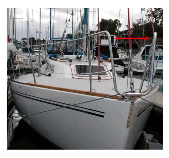
2.4.3 Bow pulpits may be open, but the opening between the vertical portion of stanchion pulpit and any part of the boat shall not exceed 14.2" (360mm).
