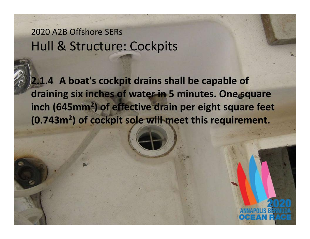
Hull & Structure: Through Hulls
